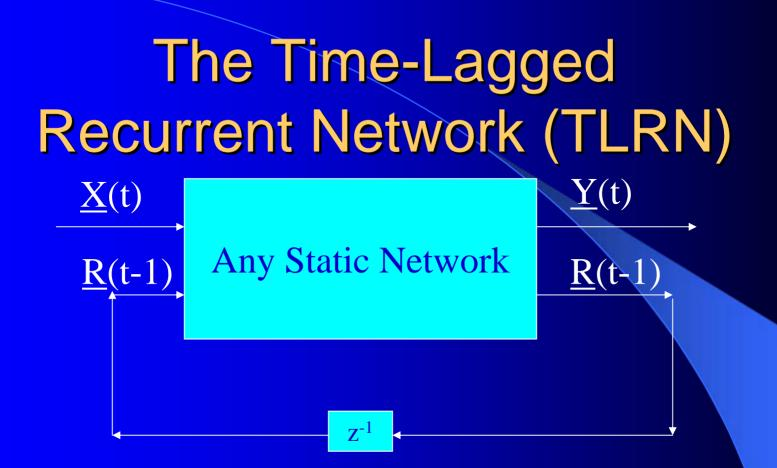
$\underline{Y}(t) = \underline{f}(\underline{X}(t), \underline{R}(t-1)); \underline{R}(t) = \underline{g}(\underline{X}(t), \underline{R}(t-1))$ f and g represent 2 outputs of one network All-encompassing, NARMAX(1 = n) Felkamp/Prokhorov Yale03: >>EKF,  $\approx$  hairy
